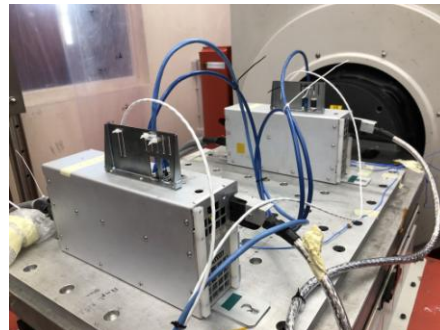
Figure 27 Assembly on vibration machine.
