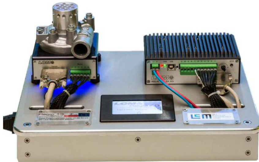
Figure 5.4.: Prototype demonstrator equipped with impeller head and housing as well as speed display and power electronic circuit
