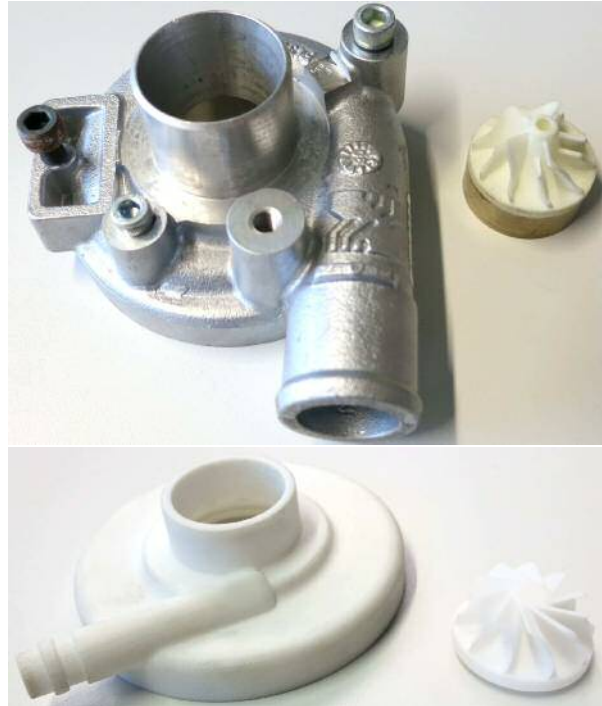
Figure 5.12.: Housing and rotor equipped with compressor wheel (top) and housing and turbine wheel ready for mounting on the same rotor (bottom)
